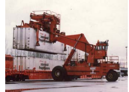
TOP LIFT EQUIPMENT
